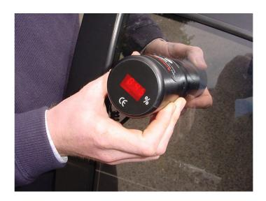
With +/- 3% accuracy, the device has a new configuration and shape (as seen in the image above), which allows easy alignment to the glass.
